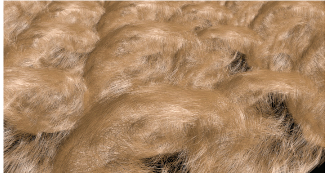
Figure 15: 430k transparent hairs ( \alpha = 0.6 , opacity threshold: 0.96) rendered at 720x389 with 8x8 sampling. This generates 43M micropolygons and 58M pixel samples in RenderMan, and condenses to 11M visible shading samples and 17M unique visibility samples through lossless visibility compression, rendering at 12 Hz and fully refining in 33 secs. Compression and performance are even better at \alpha = 1.0 , but \alpha = 0.1 (threshold: 0.996) generates 21M visible shading samples, overflowing the 16M sample textures we currently use (cf. Fig. 10).
